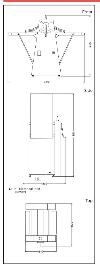
Electric Supply voltage: 230/400 V/3 ph/50/60 Hz **Total Watts:** 0.75 kW Key Information: External dimensions, Width: 2380 mm External dimensions, Depth: 890 mm External dimensions, 1265 mm Height: Net weight (kg): 179
